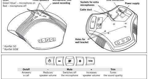
The **Konftel 50** and **Konftel 60W** are conference units for connection to an existing fixed system phone, DECT telephone, mobile phone or computer. The **USB adapter** makes it possible to connect the units to a computer that does not have a suitable sound port. The USB adapter functions as a sound card in a computer without inputs and outputs for sound. Connection with a USB adapter and its use are the same for both a Konftel 50 and a Konftel 60W.
